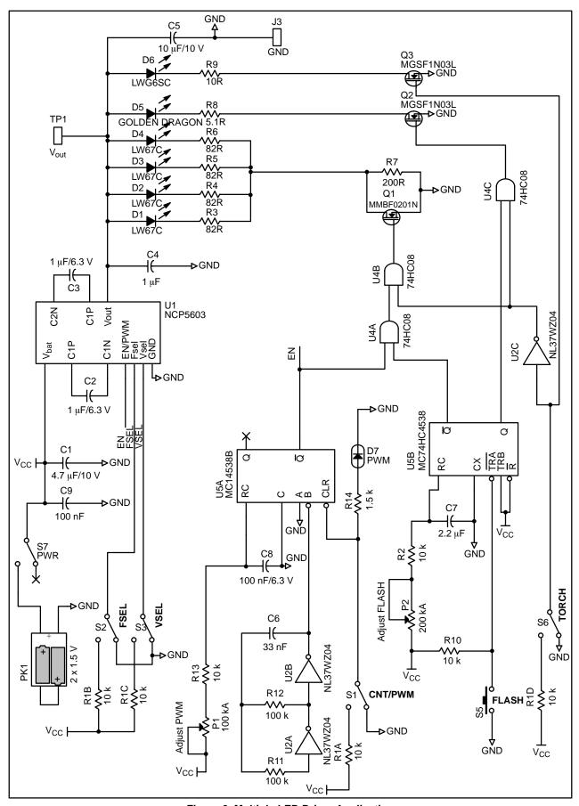
Figure 2. Multiple LED Driver Application
