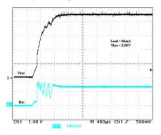
Figure 4. Typical Startup Timing
