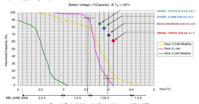
Figure 1. Typical Lithium-Ion Battery Voltage and White LED
